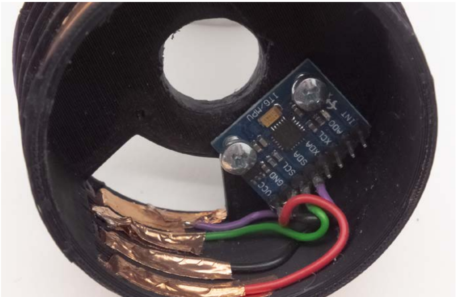
Figure 18: Slip ring, showing inside connections
