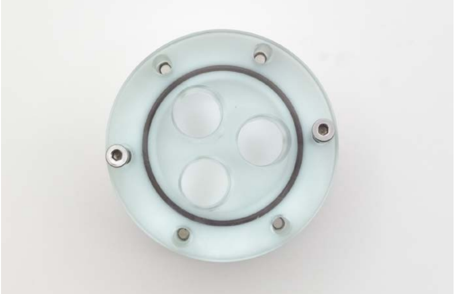
Figure 16: Vessel with glass top, partially screwed together
