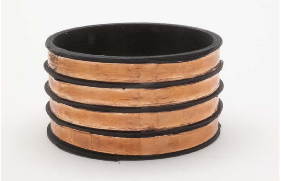
Figure 17: Slip ring, showing copper tape around circumference
