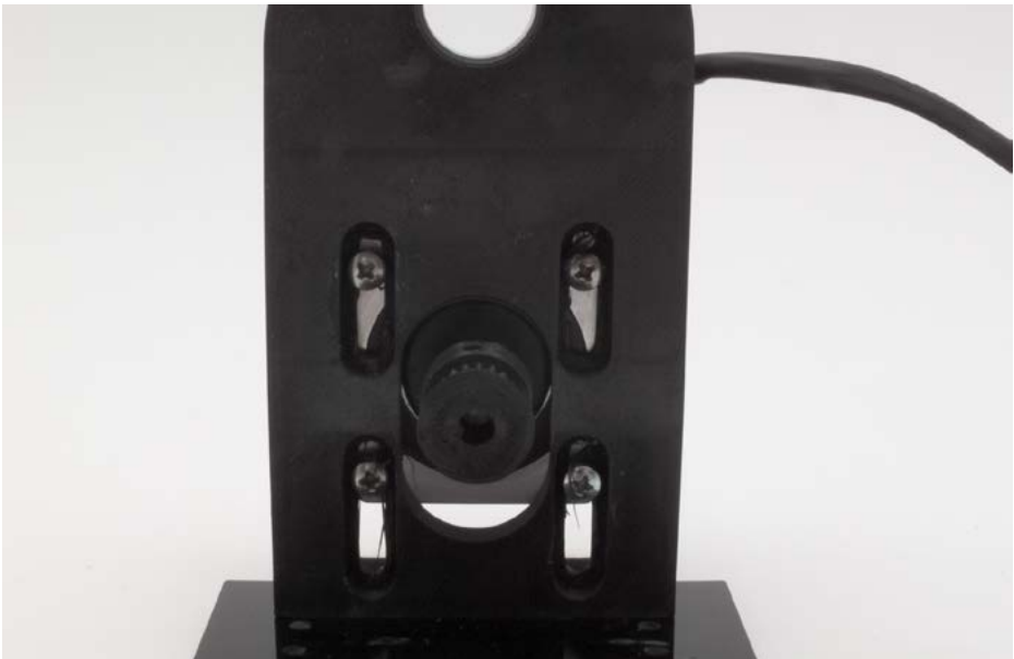
Figure 21: Small sprocket wheel and motor attached to the arm
