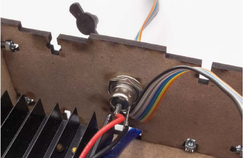
Figure 28: 5.5x2.1mm plug wiring
